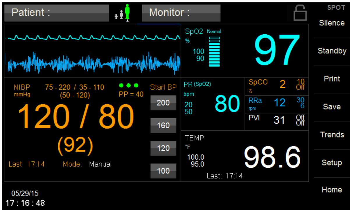
Figure 16: Main Screen w/SpCO, RRa & PVI enabled
