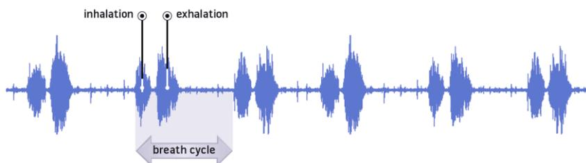
Figure 8: Acoustic signal showing several complete breaths
