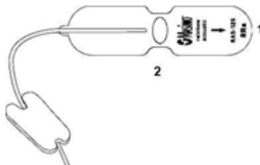
Figure 11: Acoustic Sensor
